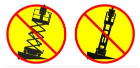
Do not depend on the tilt alarm as a level indicator. The tilt alarm sounds on the chassis and in the platform when the machine is on a slope.
