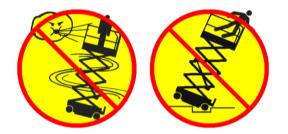
Do not use the platform controls to free a platform that is caught, snagged or otherwise prevented from normal motion by an adjacent structure. All personnel must be removed from the platform before attempting to free the platform using the ground controls.
