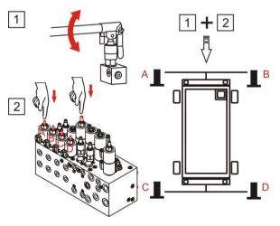
1 Unplug the lever and put it into the hand pump (1)
