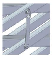
3 Lower the platform until the safety arm rests securely on the shaft. Keep clear of the safety arm when lowering the platform.
