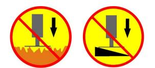
In case of special (soft or inclined) ground, the wood or steel pad suitable for the ground must be used under the support plate, and it must be firm and not cave in during the operation.
