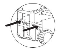
Position the forklift forks in position with the forklift pockets.
