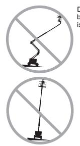
Do not raise or extend the boom unless the machine is on a firm, level surface.
