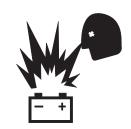
Keep sparks, flames and lighted tobacco away from batteries. Batteries emit explosive gas.
