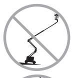
Do not raise or extend the boom unless the machine is on a firm, level surface.
