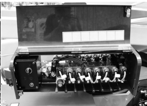
Fig. 57 Carter hydraulic control aerial part
