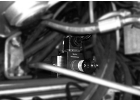
Fig. 135 Aerial-tracked part switch
