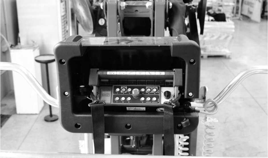
Fig. 19 Basket control protection
