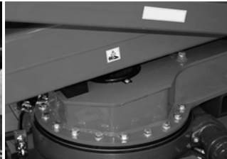
Fig. 97 Example potential shearing risk zone 2
