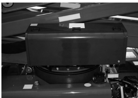
Fig. 122 Aerial part distributor protection
