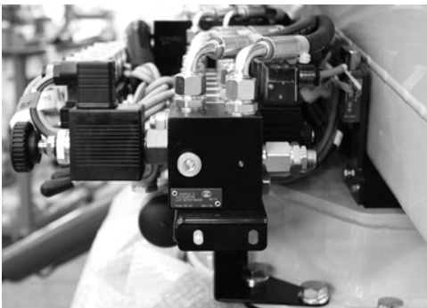
Fig. 8 Aerial part pressure relief valve
