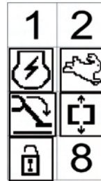
Fig. 129 Emergency BY-PASS activated
