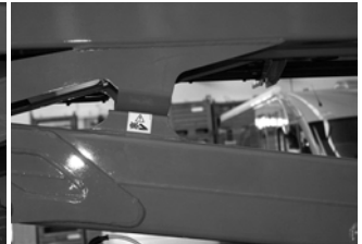
Fig. 98 Example potential shearing risk zone 3
