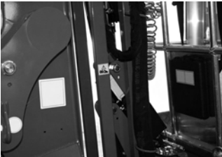
Fig. 96 Example potential shearing risk zone 1
