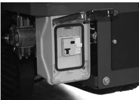
Fig. 84 Main electric switch
