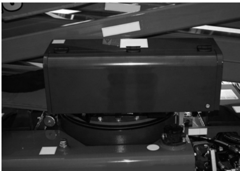
Fig. 110 Aerial part distributor protection
