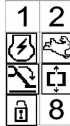
Fig. 134 Emergency BY-PASS activated
