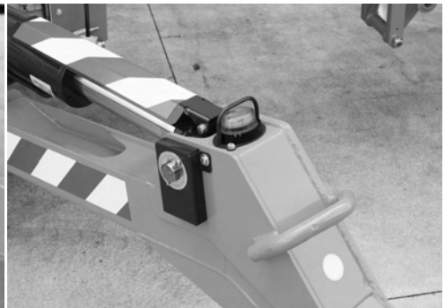
Fig. 15 Indicator light plate on the ground
