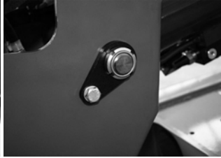
Fig. 28 Bolts to stop rotation
