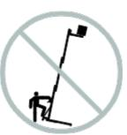
Do not operate the machine in strong or gusty winds. Increasing the load surface area will decrease machine stability in windy conditions.
