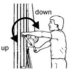
4 Lower the load by firmly grasping the winch handles and rotating them away from the mast. After lowering to the desired position, turn the winch handles toward the mast (raise the load) 1/4 turn to set the brakes.
