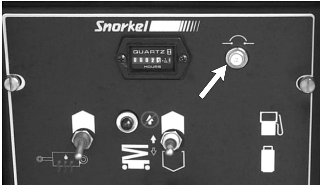
Figure 5.4 - Main Circuit Breaker
