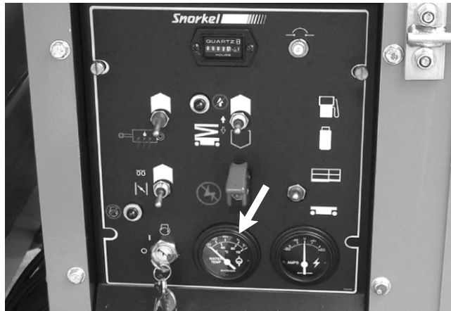
Figure 4.1 - Water Temperature Gauge
