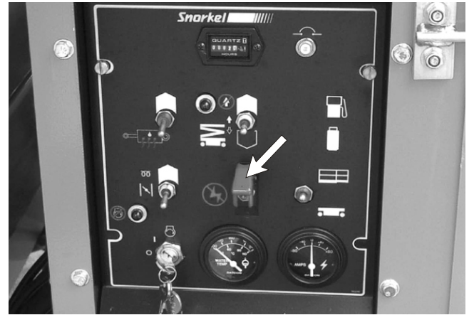
Figure 8.1 - Emergency Stop Switch at Ground Control Box
