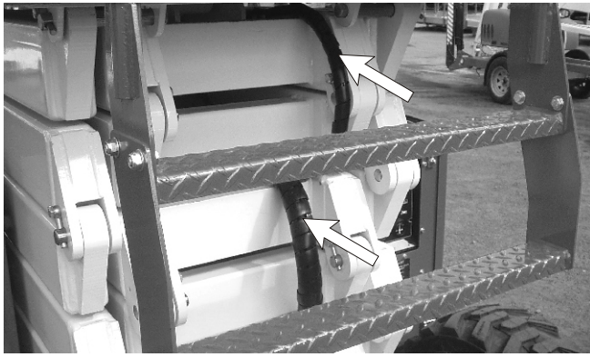
Figure 7.11 - Wiring Harness in the Scissor Stack
